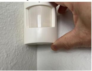
2. Locate the push tab underneath, you will need to grasp the motion with your thumb at the bottom (on tab), using your other fingers on top to squeeze the tab.
