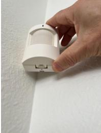
3. Remove the cover by squeezing the tab, pulling the button toward you and lifting the cover off.
