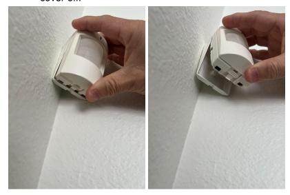
4. Remove and replace the battery (2 - AAA. Recommend Lithium). You may need a flathead screwdriver to assist you.
