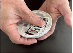
5. When placing cover back on, line up the notch on the side to the lin mark on the base. Turn the cover clockwise and the it lock in place
