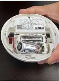
4. Please make sure the positive and negative sides are in the right position. In the photo above, the positive side is opposite of the springs. Both batteries are facing in the same direction.
