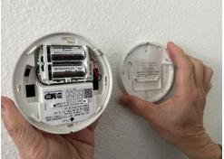
3. Remove and replace the battery (2 - CR123. Recommend Lithium). You may need a flathead screwdriver to assist you.
