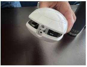
7. Close the cover and tighten the screw back in. Low battery signal will go away.
