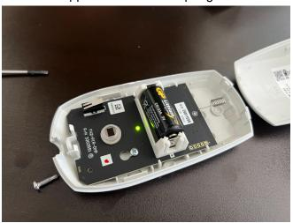
6. To place the cover back on, first put in the top side first (fitting into the notches as shown in the picture below).
