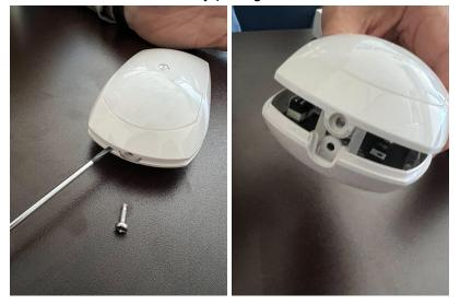
4. Remove and replace the battery (1- CR123 . Recommend Lithium). You may need a flathead screwdriver to assist you.
