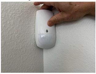
2. Locate the set screw underneath.
