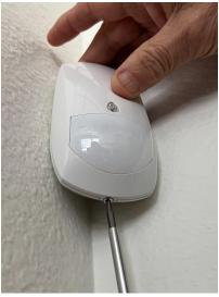
3. Remove the cover by pulling the bottom out first, make sure to not lose the set screw
