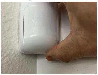
2. Locate the push tab underneath, you will need to use a flathead screwdriver to push it in. You will pull the cover toward you, bottom side first.
