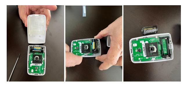
4. Please make sure the positive and negative sides are in the right position. In the photo below, the battery slot has the symbols
