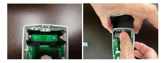
5. Place cover back on. The top side will go in first and then you will push it close to lock the cove back on. Give the system some time and it will reset the low battery.
